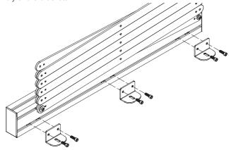
4.2 How to insert the Bosch nut into the spline
