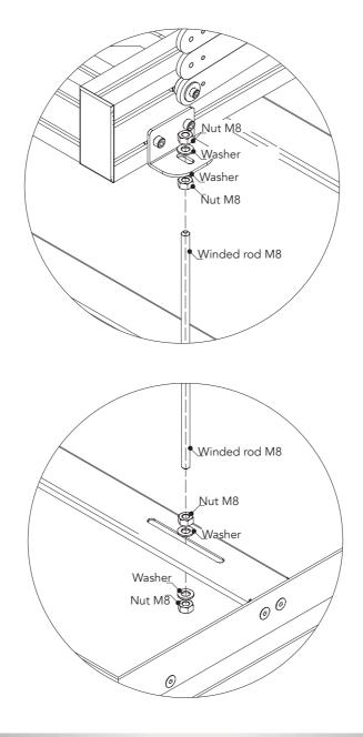
5.3 Detail of the assembled winded rods
