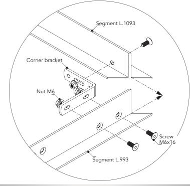
2.3 Assembly of the bezel. Once assembled the bezel, check that L1 has the same length as L2
