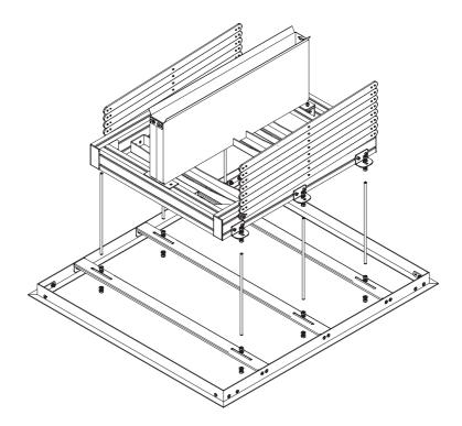
5.2 Assembly detail of the winded rods
