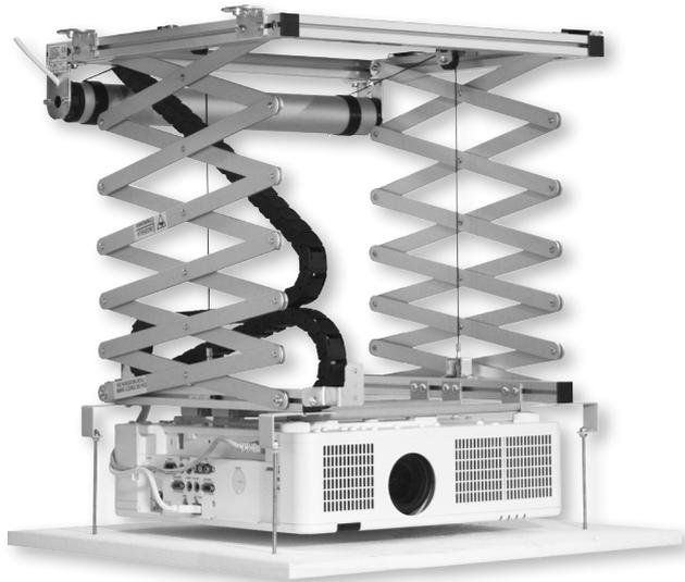
The **PROJECTOR LIFT SI-H L 200** is studied in order to support large and heavy video projectors up to 30 Kg. of weight. The SI-H L 200 is supplied with an extremely silent motor that allows a descent of a minimum of 25,5 cm. to a maximum extent of 197 cm.
