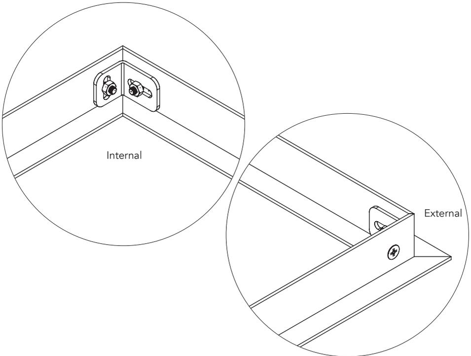
3.0 ASSEMBLY OF THE C-SHAPE PROFILES
