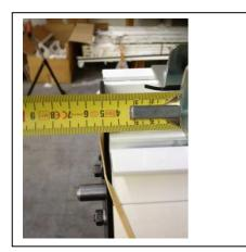
This mounting system has to be positioned at 5 cm from the end of the screen housing. See picture left.
