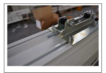
Tight or loosen the nuts at the end of the ties of the winch steel cables, in order to adjust the screen housing perfect horizontally.
