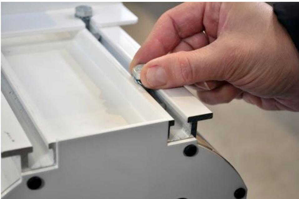
At this point, insert in the housing splines, for each mounting bracket two sets of bolt, washer and nut.
