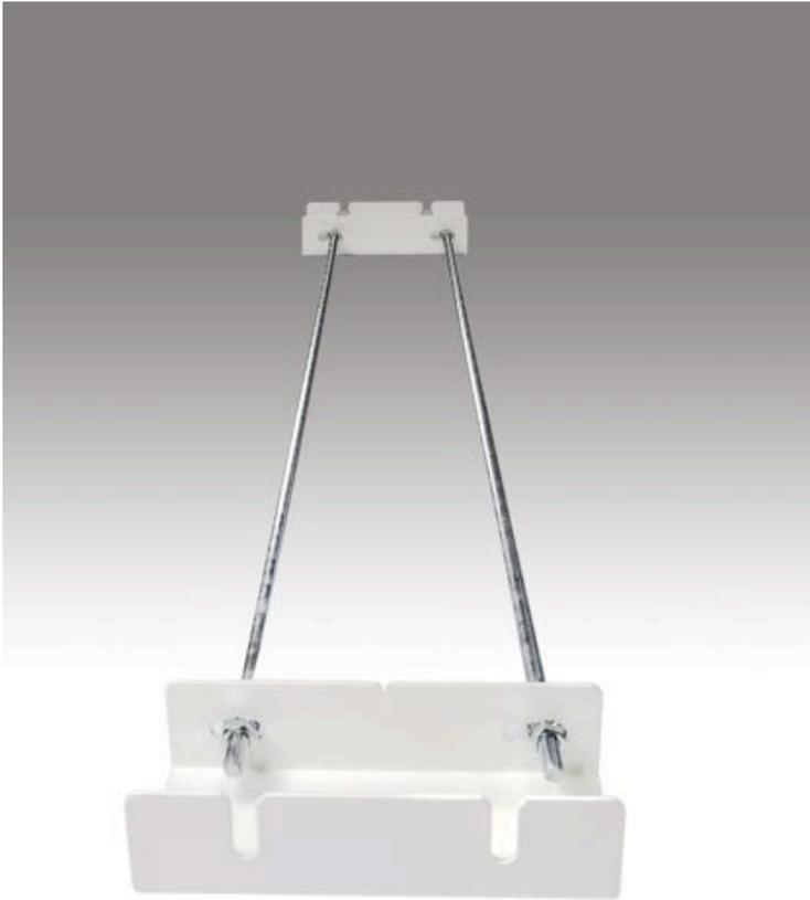
Fix the lower bracket to the end of the metal rods taking care that at least 3 cm. of metal rod goes inside the bracket.
