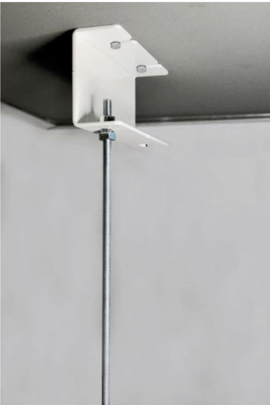
Cut the metal threaded rods at the desired length, taking care that the metal rod has to go inside the top and the bottom mounting bracket, at least 3 cm.
